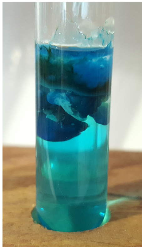
Figure 1.3: Formation of \text{Cu}(\text{OH})_2 precipitate in a test tube. Photograph by José Furtado, distributed under a CC BY-SA 4.0 license [40].
