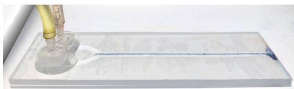
Figure 4.1: Microfluidic setup for precipitate reaction. Ionic species enter the tubes on the left, and exit the channel on the right. Reproduced from [109] with permission.
